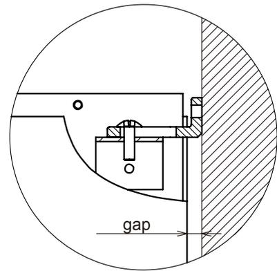
\* When you fix the basin body on the wall with no gap and inclined wall, the basin body will be fixed improperly. The gap between basin and basin body will vary.
