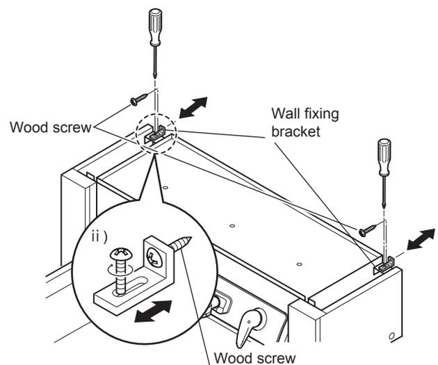
\* If there is gap between the basin body and the wall, fix the basin body on the wall keeping gap.
